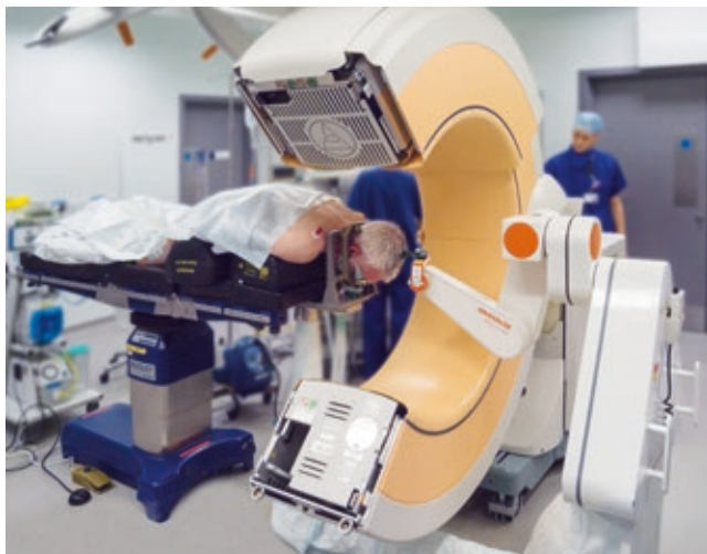
The neuromate stereotactic robot in use with a neurolocate module that is mounted to the robot to register a patient's position using either computed tomography (CT) or X-ray.
